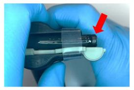
**6** Aligning the Transducer on the same side as the endoscope's UP angulation will provide optimal ultrasound coupling.
